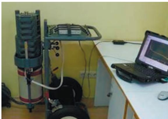
Fig. 3. Gamma radiation spectrometer (CANBERRA, USA)
